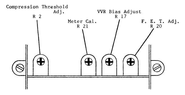
2. Set CLA-40 controls as follows: Meter Switch to +10 VU, Compress/Limit Switch to compress/limit out, Input Lever Control to maximum clockwise position, Output Level to maximum counter-clockwise position, Input Pad to "O" DB, AM-FM Switch to SYM position.
